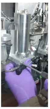
10.1.2 Place cylinder on bench as seen below. Take caution as there will be glue that can spill onto unprotected surfaces. Unscrew nut at the head of cylinder.
