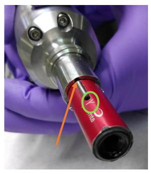
10.2.5 Screw the bottom cylinder back in, make sure to align correctly the two parts (orange rectangle). A small gap is normal so that the red stator is visible.
