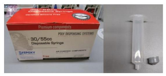
6.3.1 Label each filled syringe with the Lot Number(s) of the resin and hardener used. CAUTION: Don't fill higher than 2 cm from the top edge of the syringe.
