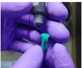
3.2.4 Remove the impeller portion from the mixing chamber and then use a pipe cleaner to clean the chamber through the feeder holes and under the impeller blades.
